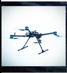
The integration of a lightweight and integrated sensor kit (inertial and Lidar) on SIGMA's drones aims to develop reliable and highperformance autonomous navigation tools. SIGMA's innovative drones include Horus, Helyx-Zero, and Helyx-One. Horus, with a payload capacity of up to 10 kg, is designed for 3D laser reconstructions and autonomous missions using Al-based navigation algorithms. Helyx-Zero, a light and compact 3D-printed drone, is ideal for surveys and precision agriculture.
