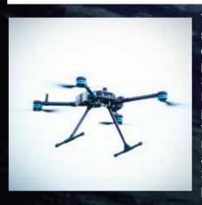
The integration of a lightweight and integrated sensor kit (inertial and Lidar) on SIGMA's drones aims to develop reliable and high-performance autonomous navigation tools. SIGMA's innovative drones include Horus, Helyx-Zero, and Helyx-One. Horus, with a payload capacity of up to 10 kg, is designed for 3D laser reconstructions and autonomous missions using Al-based navigation algorithms. Helyx-Zero, a light and compact 3D-printed drone, is ideal for surveys and precision agriculture.
