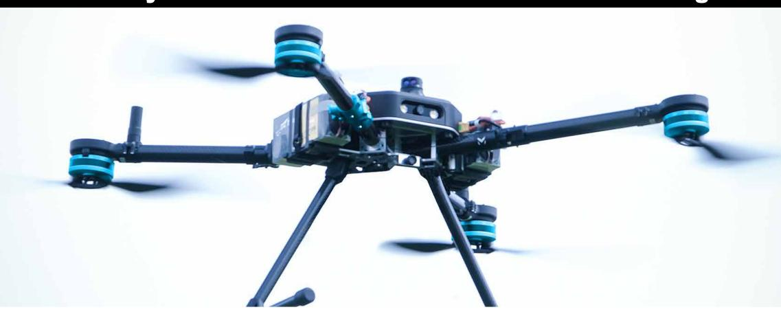
The integration of a lightweight and integrated sensor kit (inertial and Lidar) on SIGMA's drones aims to develop reliable and high-performance autonomous navigation tools. SIGMA's innovative drones include Horus, Helyx-Zero, and Helyx-One. Horus, with a payload capacity of up to 10 kg, is designed for 3D laser reconstructions and autonomous missions using Al-based navigation algorithms. Helyx-Zero, a light and compact 3D-printed drone, is ideal for surveys and precision agriculture.
